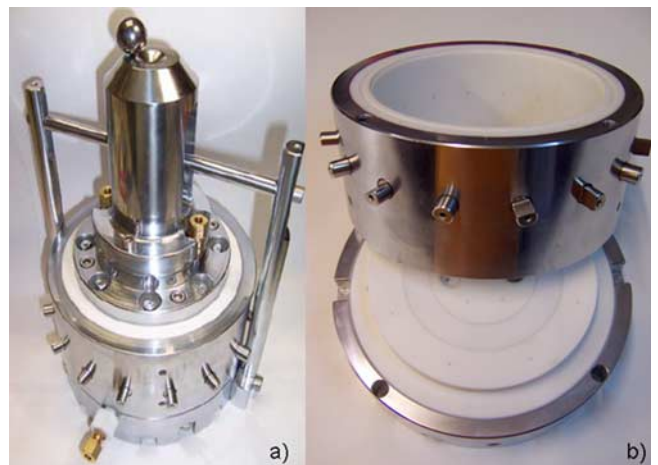
FIG. 2—EIT oedometer cell: (a) external view of the cell and loading system and (b) particulars of metallic confining ring and insulating internal material.
