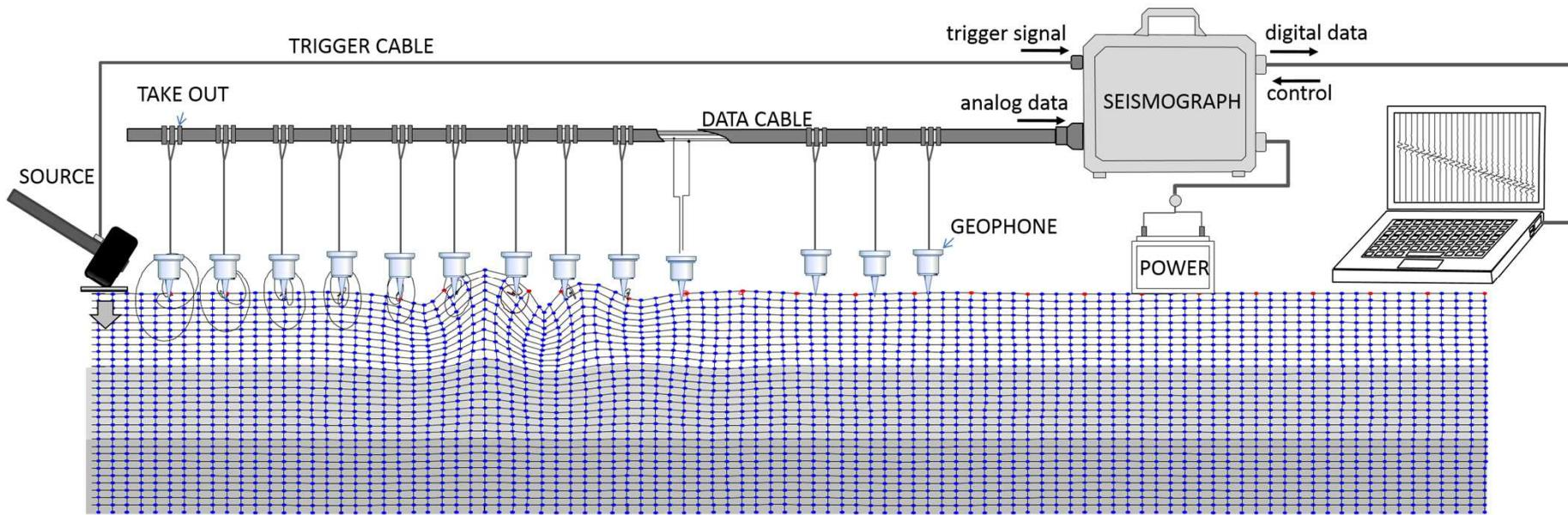
The equipment necessary for a seismic survey is:
