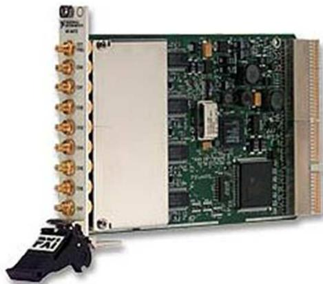
NI PCI Dynamic signal acquisition board (8 channel, 24bit, simultaneous acquisition, antialias filter)
