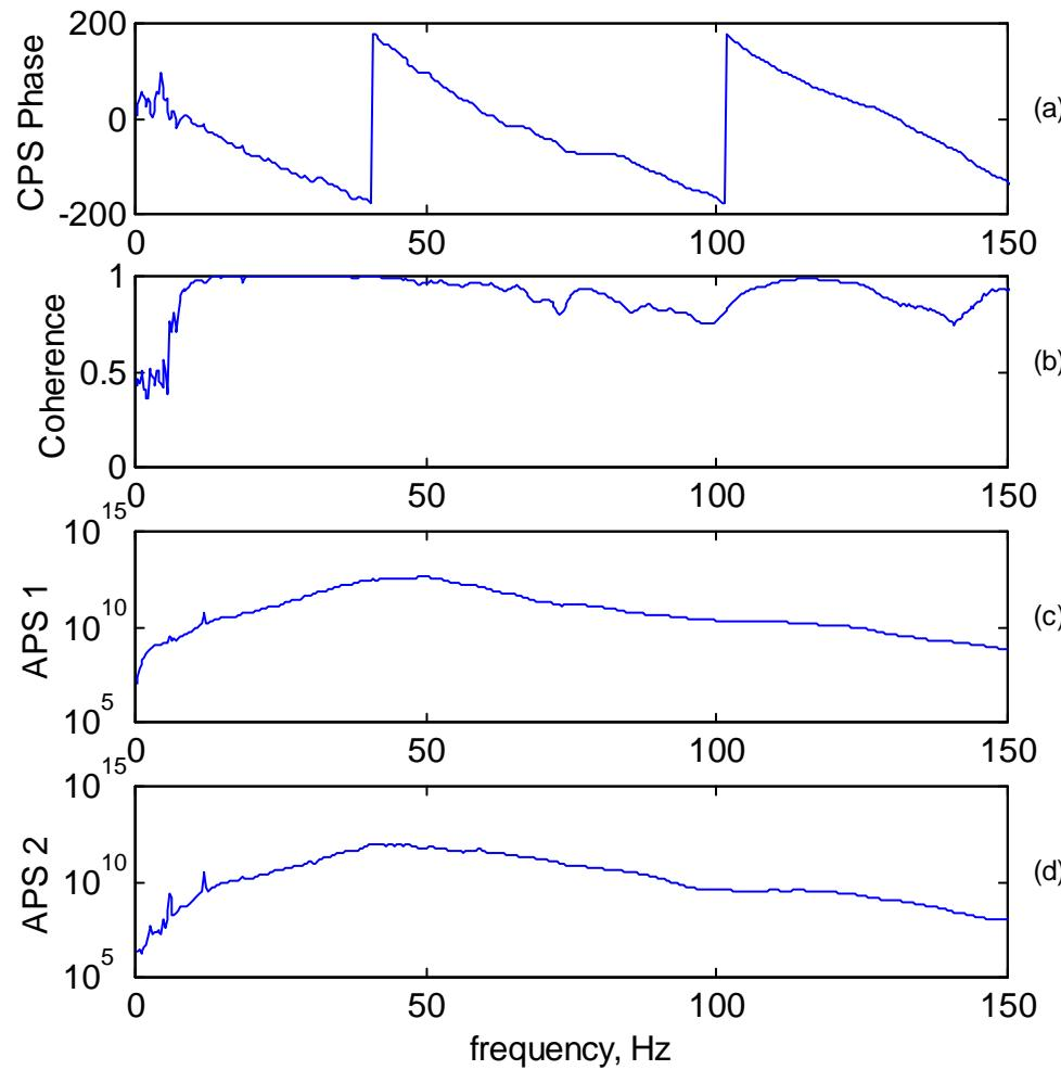
$$\Theta_{12}(\omega) = \tan^{-1} \left( \frac{\text{Im}(G_{12}(\omega))}{\text{Re}(G_{12}(\omega))} \right)$$
