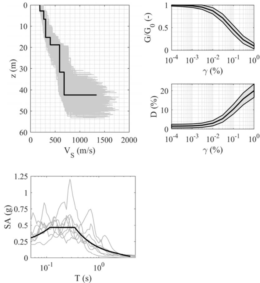
This example shows the effect of uncertainties on the site response, with focus on the role of site characterization ( $V_S$  profile from field tests and MRD curves from the lab)
