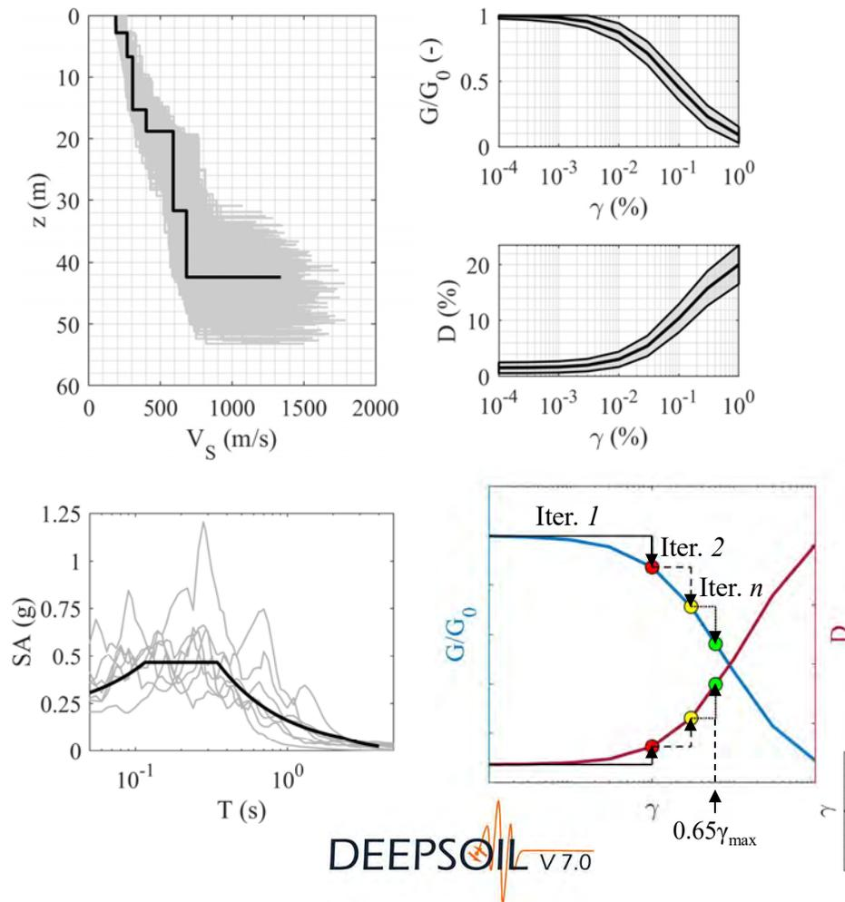
This example shows the effect of uncertainties on the site response, with focus on the role of site characterization ( $V_S$  profile from field tests and MRD curves from the lab)
