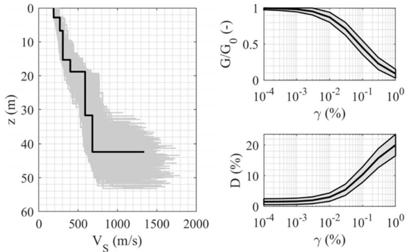
This example shows the effect of uncertainties on the site response, with focus on the role of site characterization ( $V_S$  profile from field tests and MRD curves from the lab)
